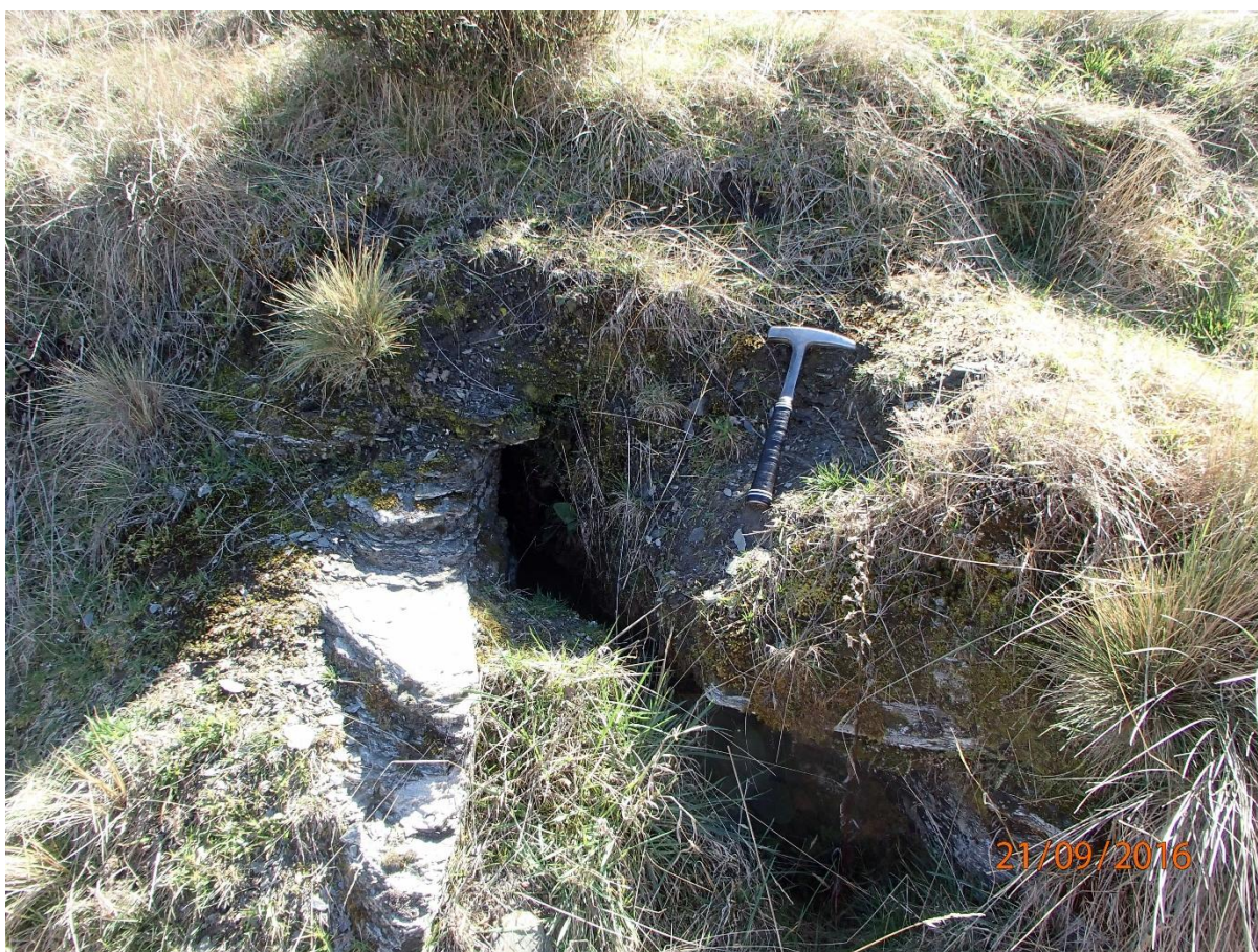
Photo 1: Open fissure in the landslide debris upslope of the proposed development.
