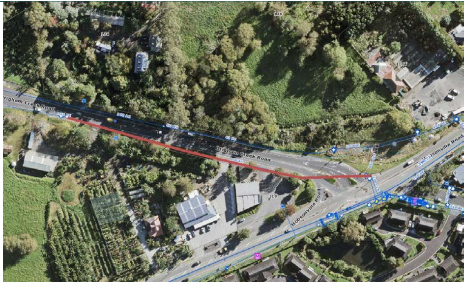
Figure 1: Proposed section of 150mm watermain to be upgraded
