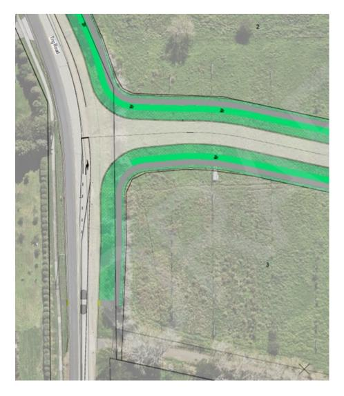
Road widening will be from the existing concrete channel on the opposite side of the road and will be enabled by vesting land along the frontage of the subject site (see proposed **46528-DR-PLN-1200-A Scheme**). A building line restriction has been shown on Lots 1 & 3 to accommodate the proposed SGA alignment for Trig Road that we request you reconsider.
