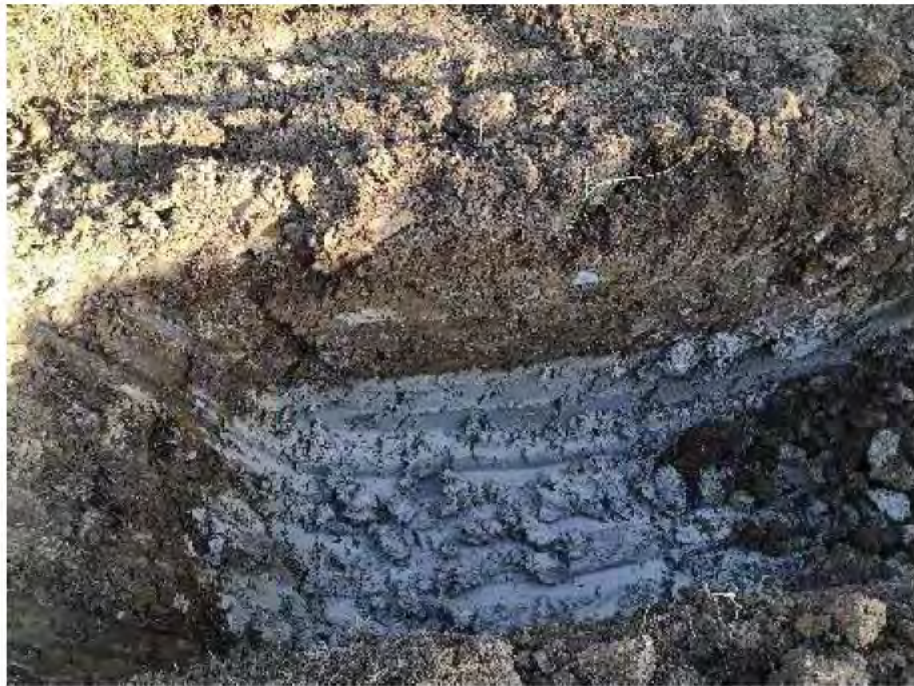
PLATE 7: shallow fill overlying natural Puketoka formation
