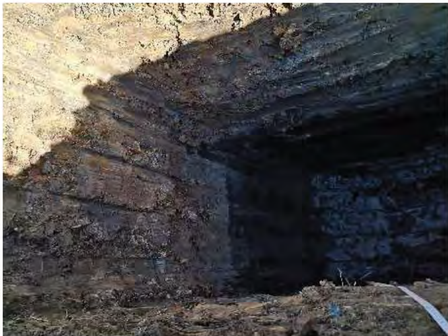
PLATE 6: indicative cross section of fill
