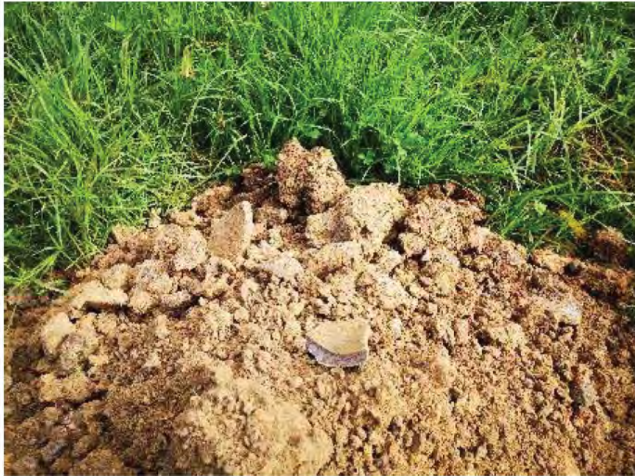
PLATE 9: ACM pipe fragment from TP11
