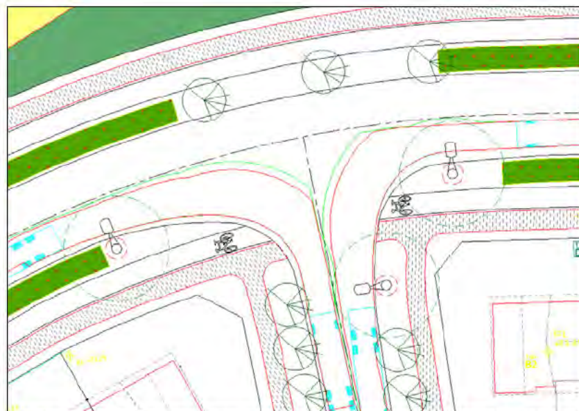
Figure 21: Large Rigid Truck Tracking Curve Plan (Main Access Road / Residential Street Intersection)
