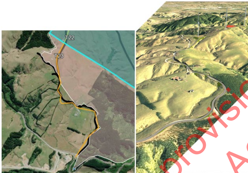
Figure 2: North Range Road Upgrades (note: the black line shows the proposed road upgrades, the yellow line shows the new Vestas road alignment, and the white line shows the local authority boundary (which largely follows North Range Road))
