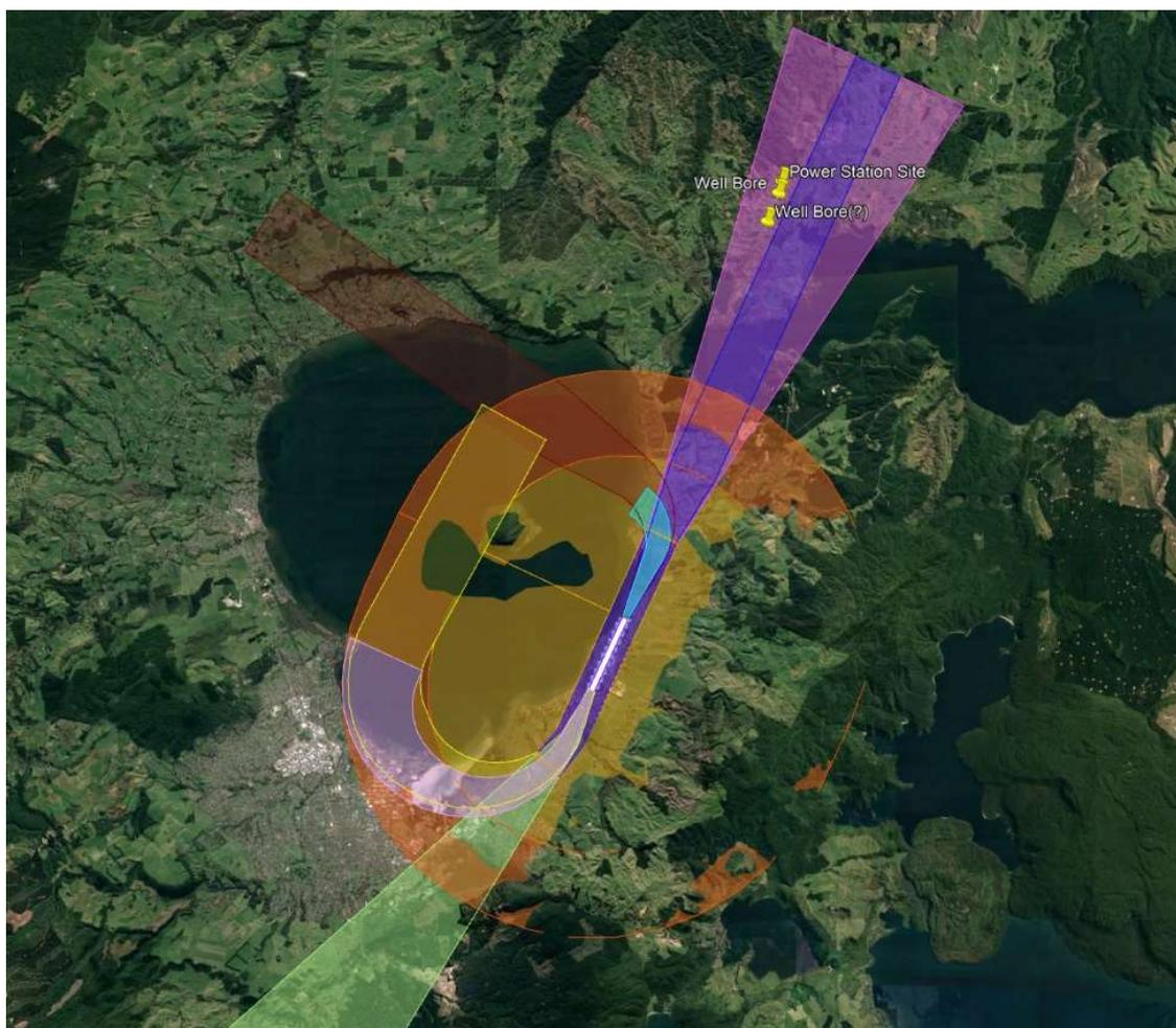
**Figure 3: Approximate Obstacle limitation surface for Rotorua Airport as provided by Rotorua Airport Limited.** The height of this surface above ground for the closest bore site is 172 m.
