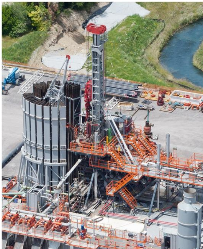
Figure 4: Photo of Rig 32 which has hydraulically controlled drill processes and has operated at the Taheke site previously.
