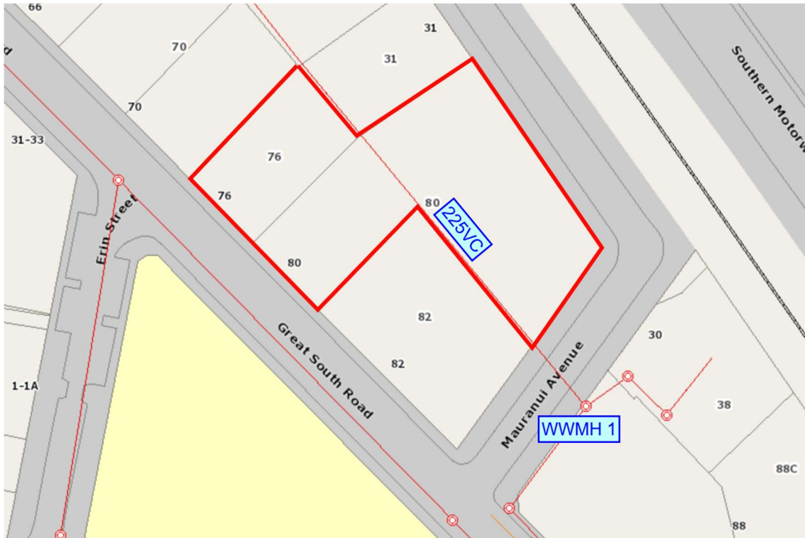
FIGURE 5-1: EXISTING WASTEWATER INFRASTRUCTURE - WATERCARE GIS
