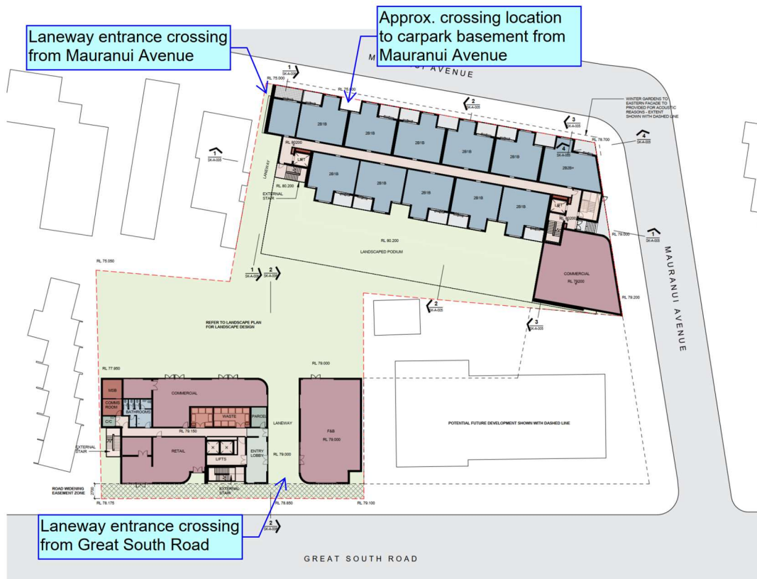
FIGURE 3-1: VEHICLE CROSSING LOCATIONS - JASMAX ARCHITECT'S EXTRACT
