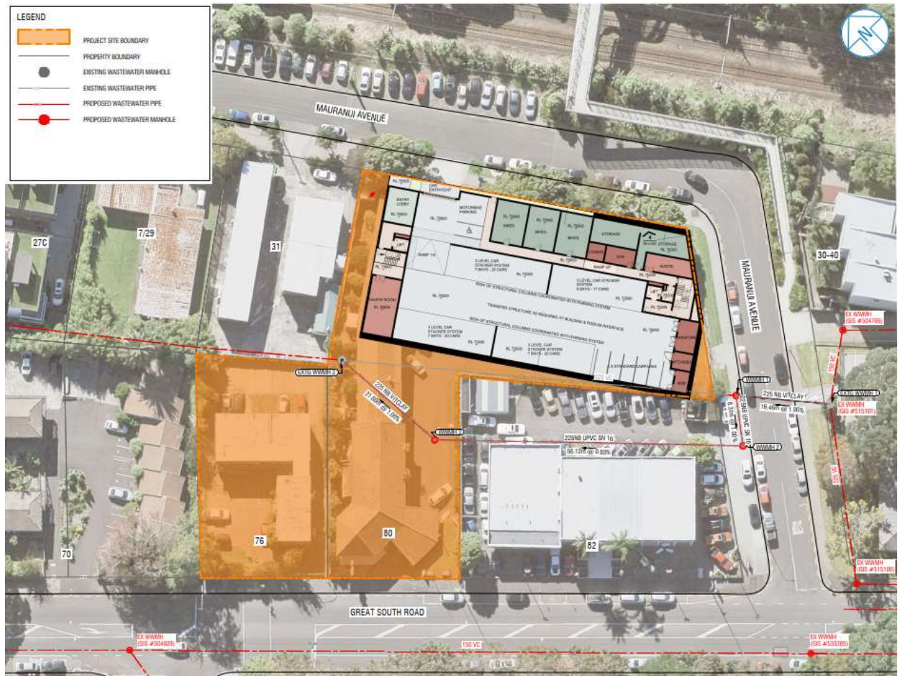
FIGURE 5-2: PROPOSED WASTEWATER LINE RELOCATION
