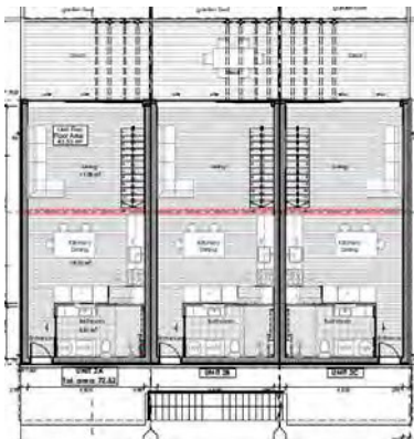
Urban Cocoon, Christchurch – Production anticipated late 2023. Three story apartment building with six units. CLT floors, HENZ walls and roof.
