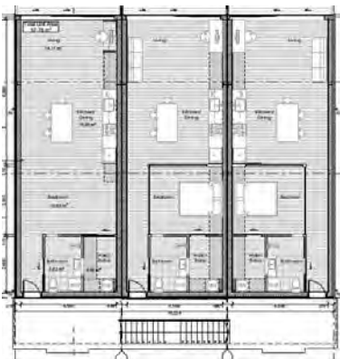
Urban Cocoon, Christchurch – Production anticipated late 2023. Three story apartment building with six units. CLT floors, HENZ walls and roof.
