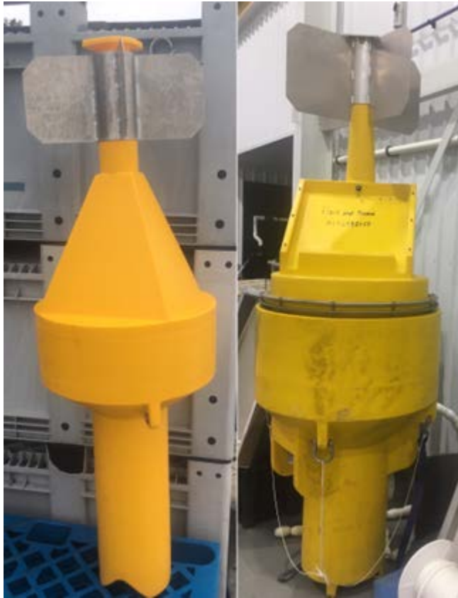
Figure 3: Examples of two large special marks appropriate for the permanent navigational marking of the mooring and associated structures. Note, radar reflectors have been added to the buoys, while lights have been removed for storage purposes
