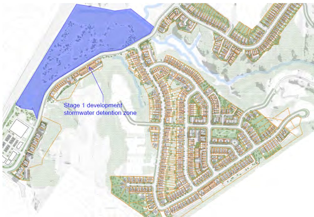
Figure 11: Stage 1 development proposed enhanced stormwater detention zone
