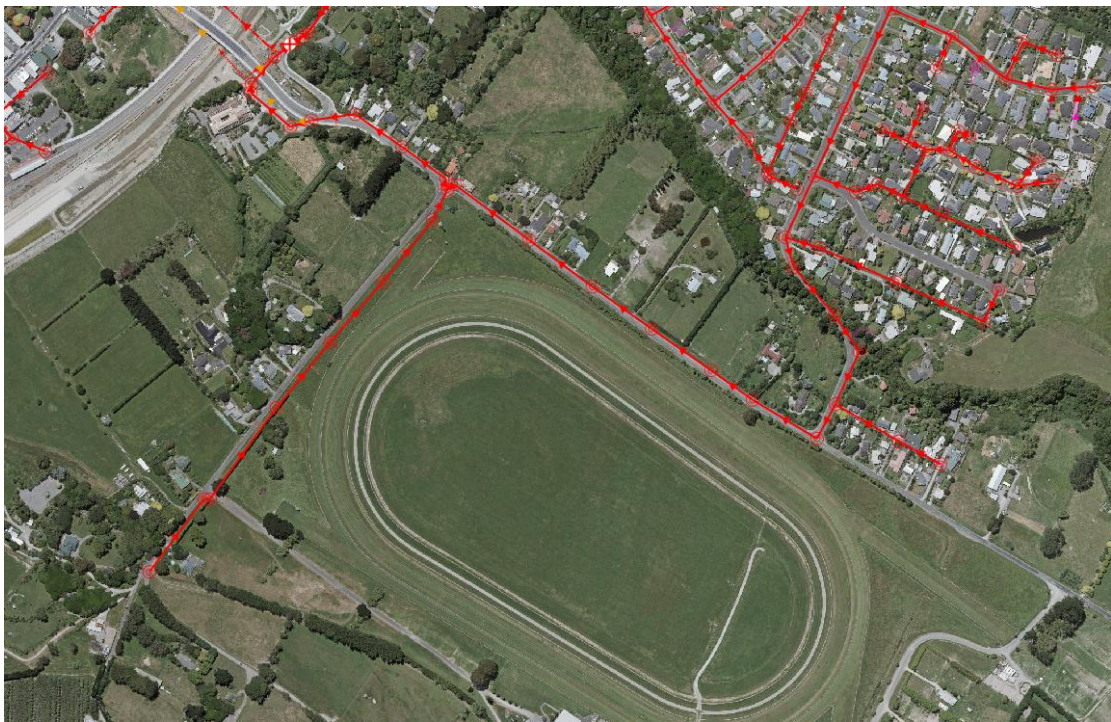
Figure 3. Wastewater network connectivity of the site
