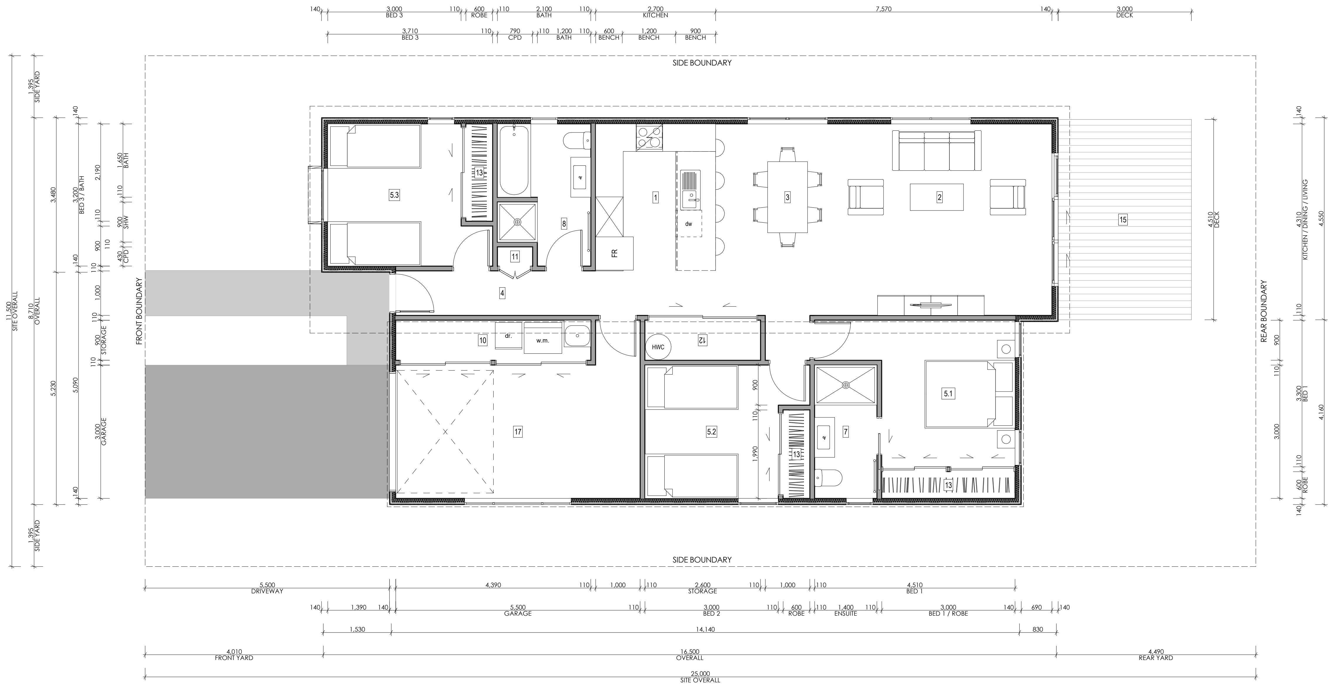
1 Type 1A - 3 Bed Standalone - Front Entry and Parking Scale 1:50
