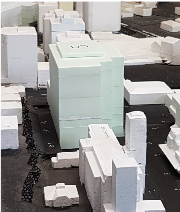
5 STEPPED CORNER • Reduces area of facade to the south, reducing downward wind hitting facade • Open corner allowing wind to dissipate
