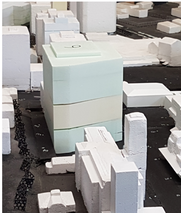
6 CHAMFER • Reducing area at of southern face, reducing downward wind hitting facade • opening up corner
