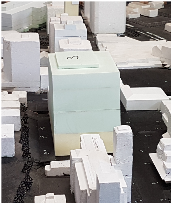
3 SLOPE • Encourages wind hitting sloped facade to drive upwards rather than to ground • Highly dependent on slope angle.
