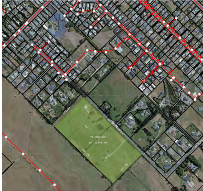
Figure 2: Existing public wastewater network
