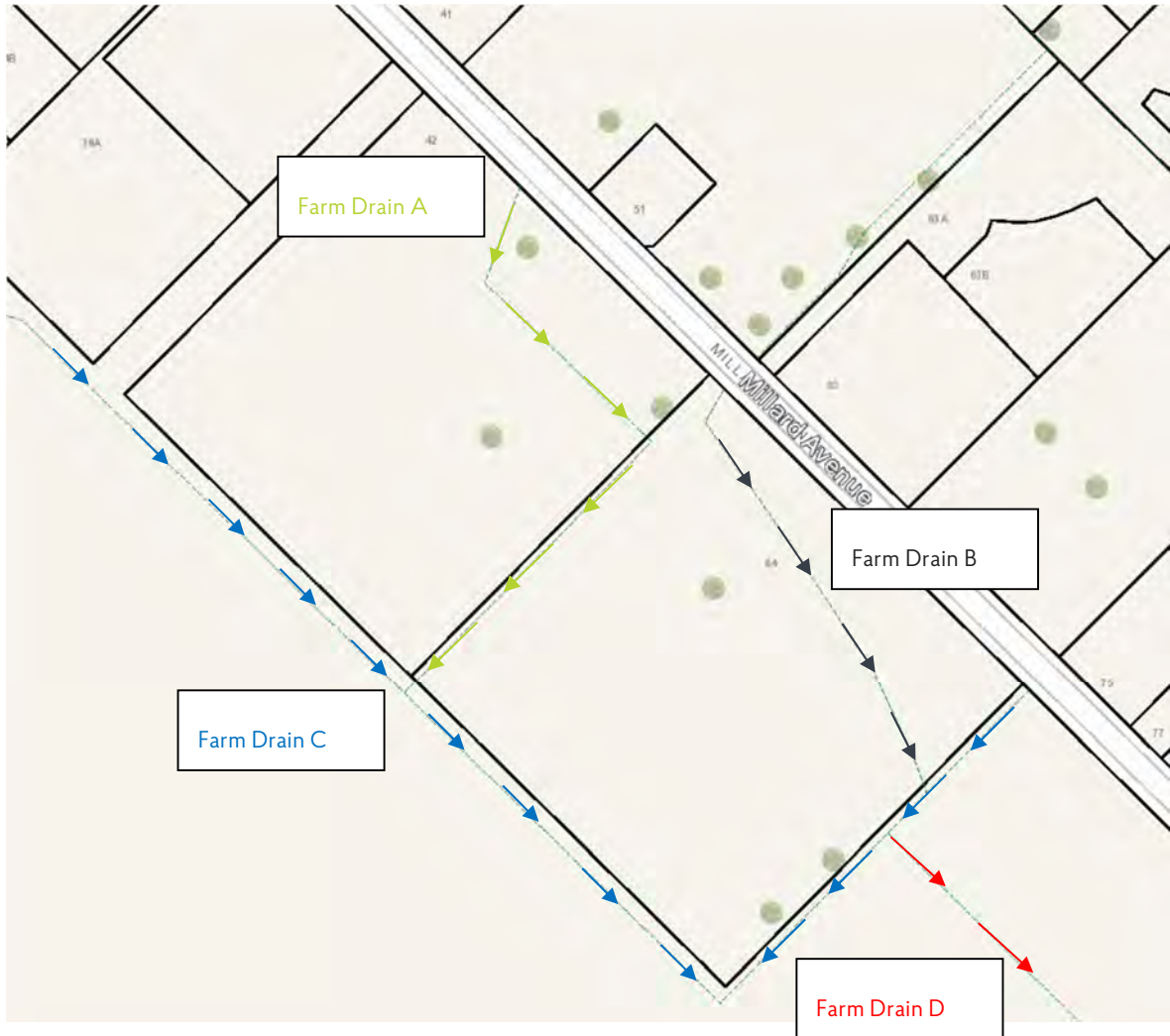
Figure 4: Existing Stormwater discharge scenario (as per Lidar)
