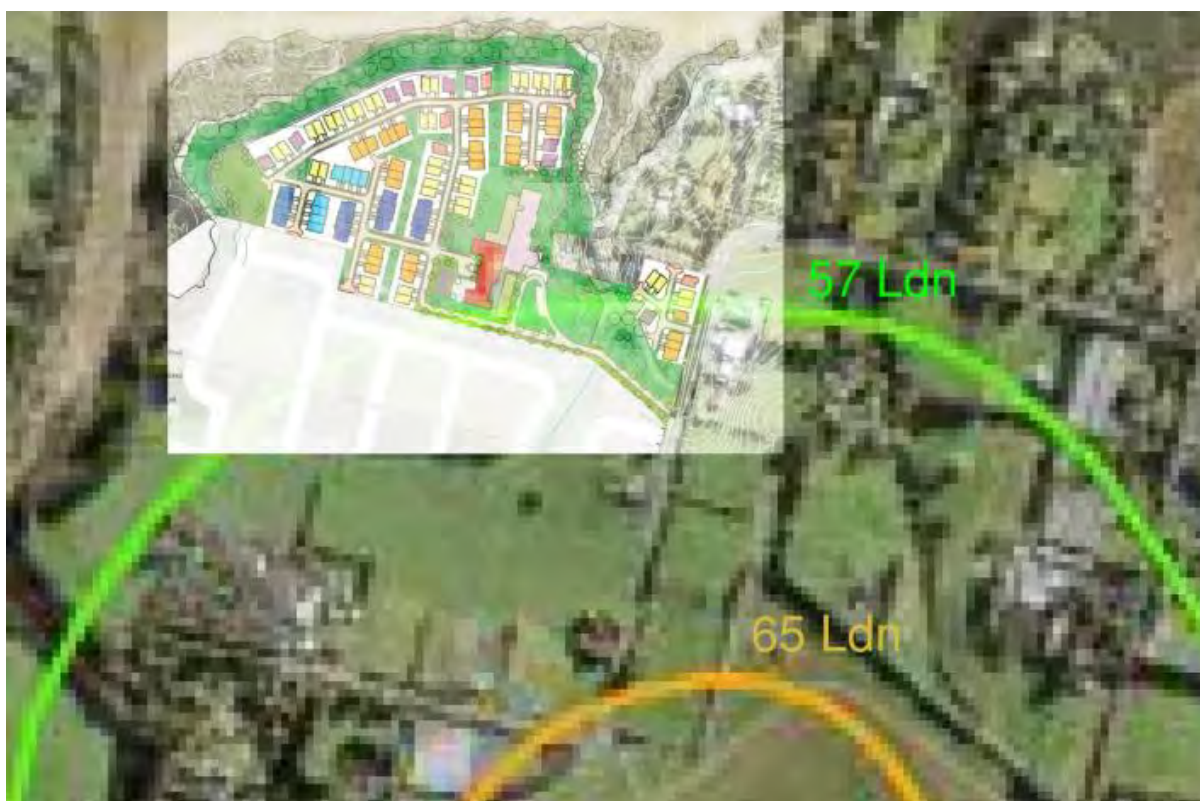
Figure 7: Engine noise testing contours in relation to the site
