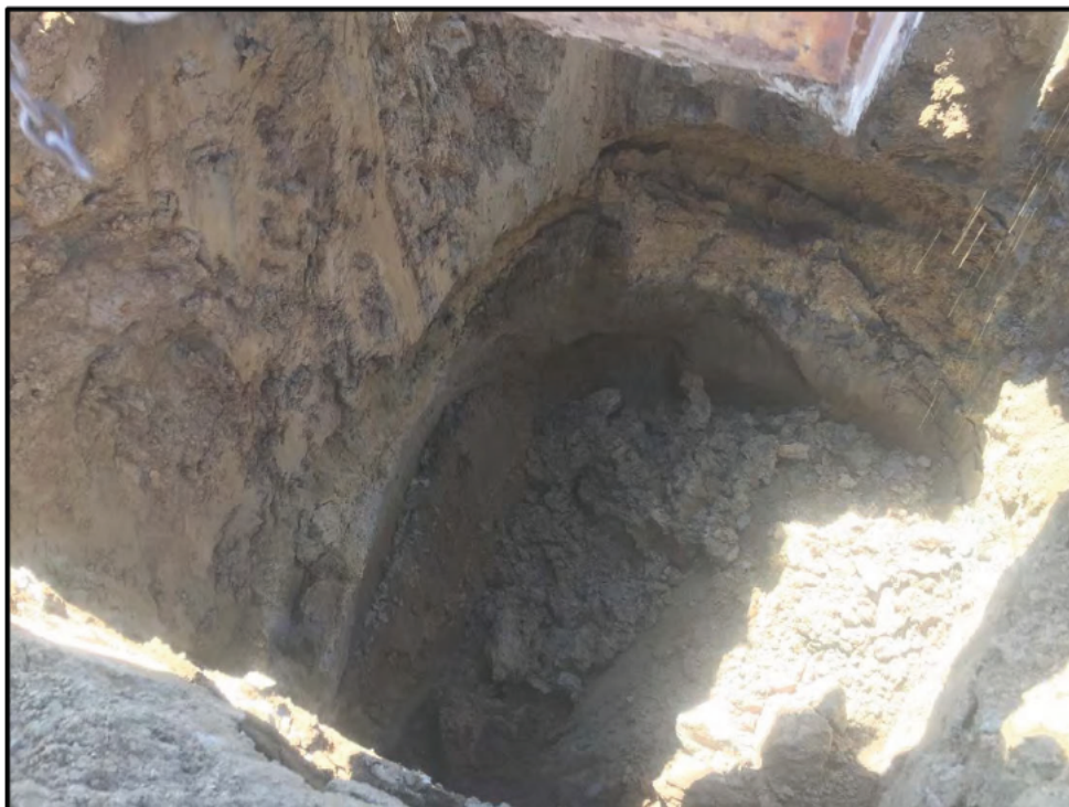
Figure 2: Photograph of a deep excavation in the pond area north of the subject area showing interbedded silt and sand deposits to at least 3.7 m below ground level
