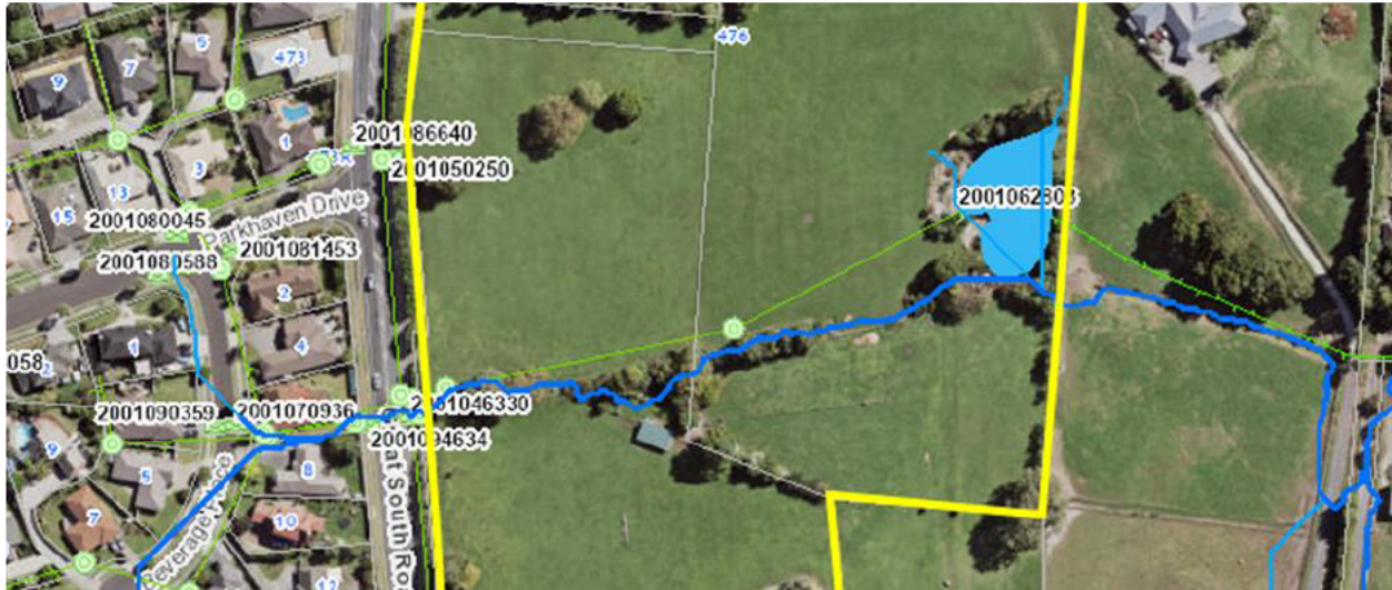
Figure 3. Auckland Council GeoMaps Underground Services Stormwater overlay illustrating the piped network to the stormwater pond (green).
