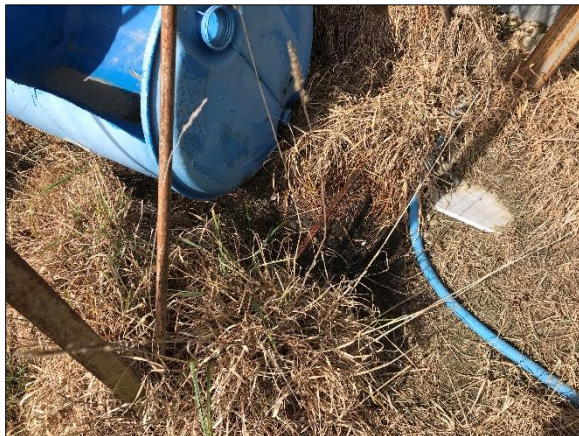
Photo 4: Staining below above ground storage tank
