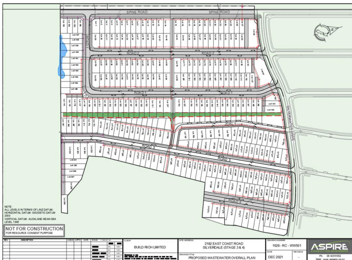
Figure 4: preliminary wastewater network layout
