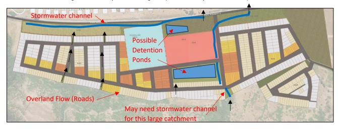
Figure 5-8: Preliminary Concept for Stormwater Quantity Management
