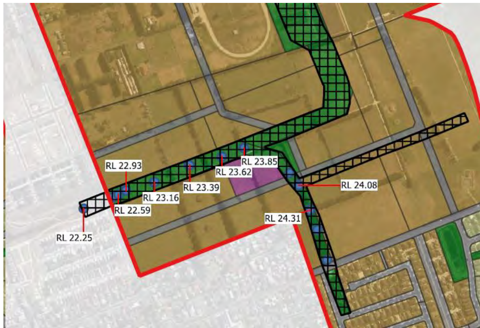
Figure 3.3 Initial Water Surface Elevation (permanent water level)
