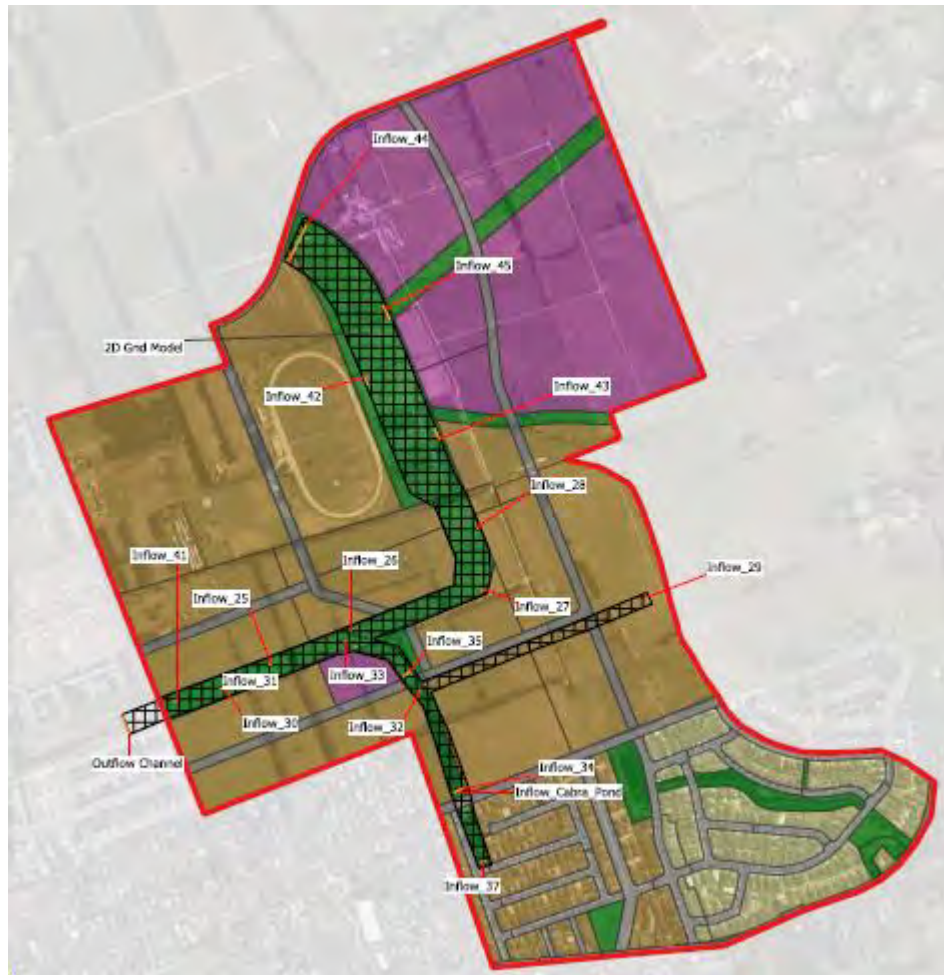
Figure 3.1 – HEC-RAS Post development Western model set-up
