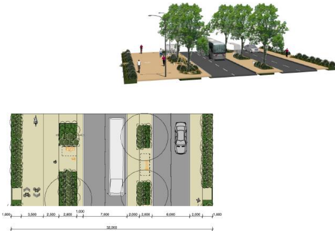
Figure 4-3: Indicative Loop Road cross section
