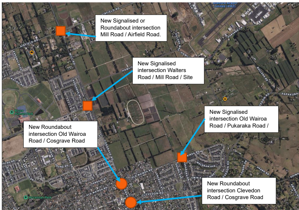
Figure 6-3: External intersection upgrades
