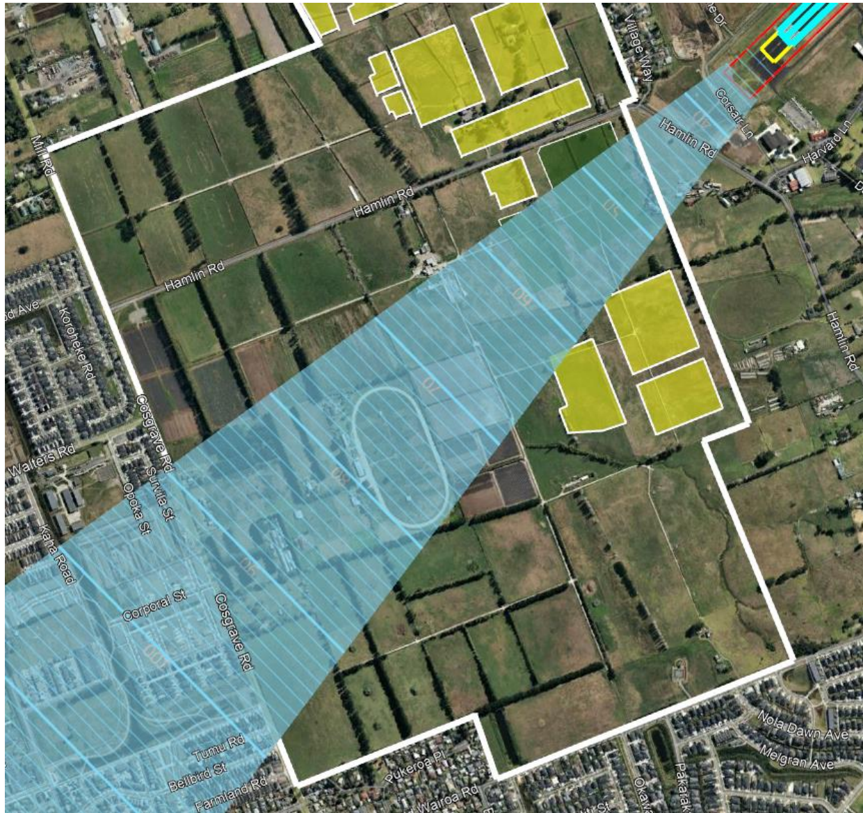
Figure 9: VSS surface for runway 03 – 52m AMSL (20m AGL) buildings not intruding
