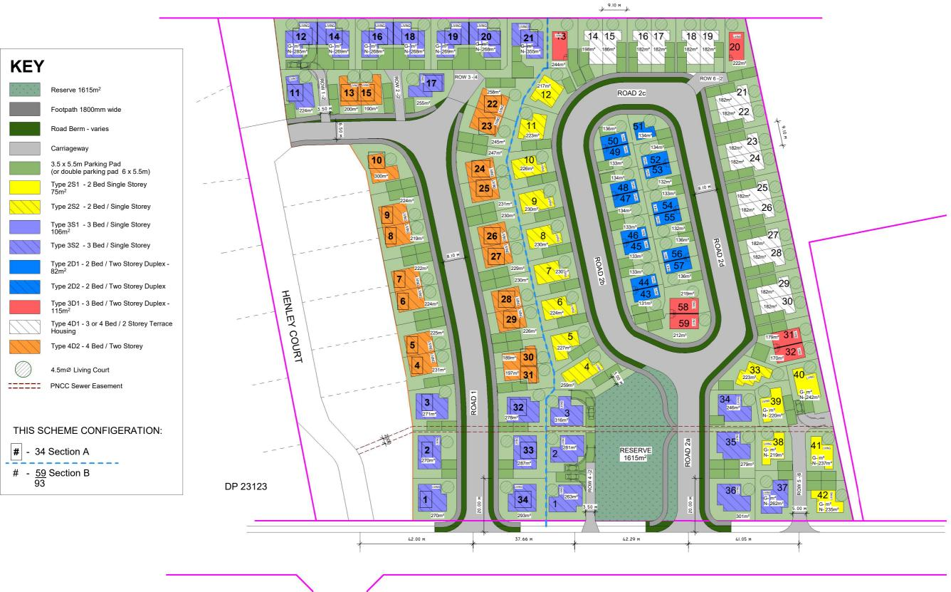
The proposed layout is subject to land use consent from PNCC. 2. A B85 percentile car with 5.8m turn radius as per NZS 2890.1:2004 has been relied on for the vehicle turning for the proposed layout.
