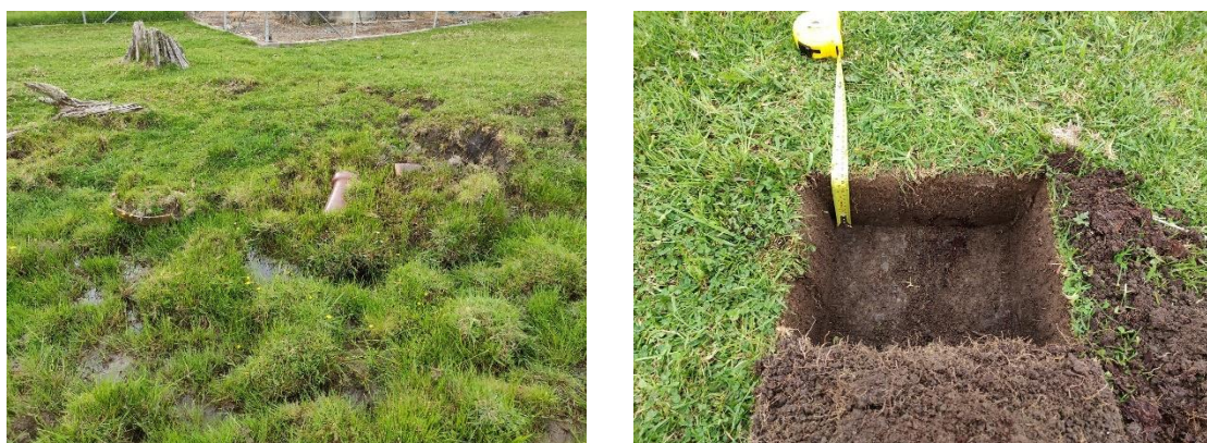
Figure 21. Unmarked glazed ceramic drainage found across northern end of south-eastern creek of 102-102A Totara Road, facing southeast (left); and test pit placed near south-eastern creek of 102-102A Totara Road. Note organic material (roots) rotting at base and in profile, facing northwest (right)
