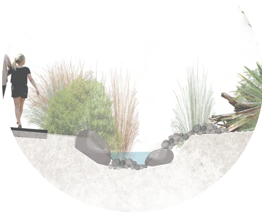
3. DRAINAGE CROSS SECTION SHOWING VARIED BANK FEATURES (to be confirmed with ecologist)
