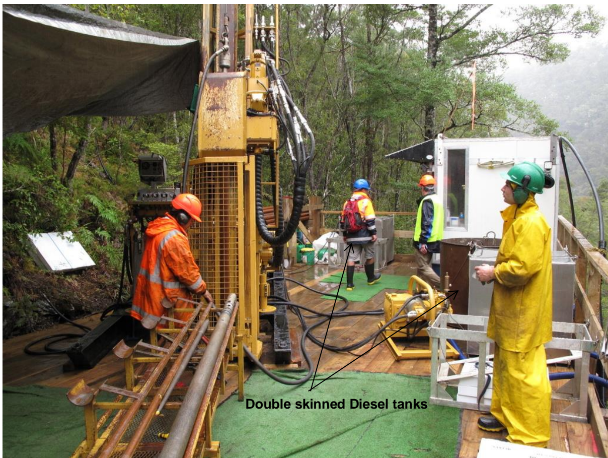
Figure 18. Stainless steel double skinned diesel containers as indicated.
