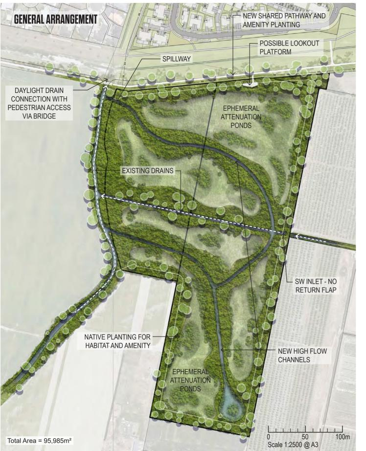
**STORMWATER FLOW DIAGRAM** LOW FLOW HIGH FLOW CULVERT CULVERT WITH NO  $\mathbf{\nabla}$ RETURN  $\Pi\Pi\Pi\Pi$ BATTERS INUNDATION BACK FLOW В
