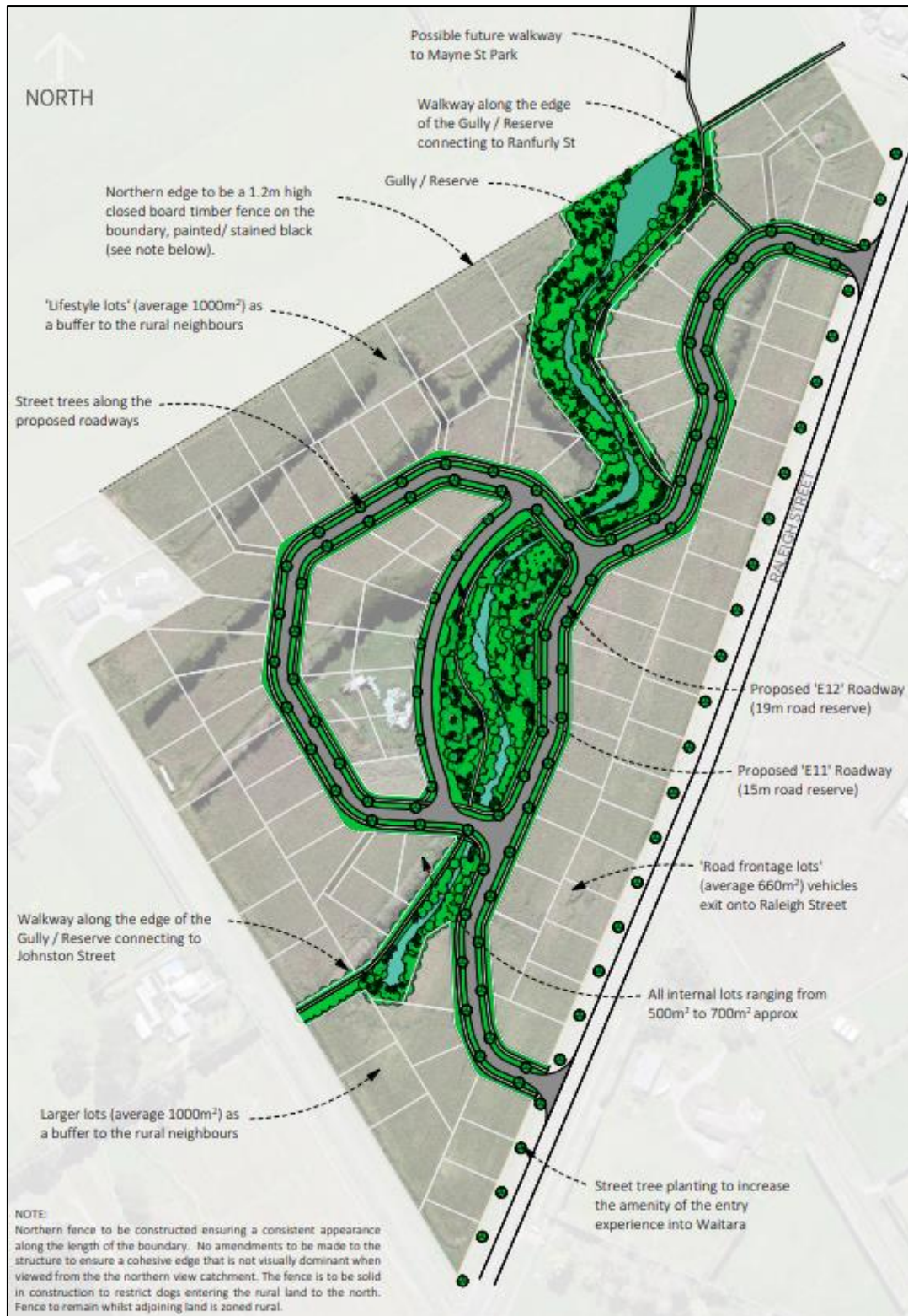
Figure 2: potential subdivision layout showing proposed Open Space Zoning, roading alignment, with the remainder being Residential A Environment Area 4
