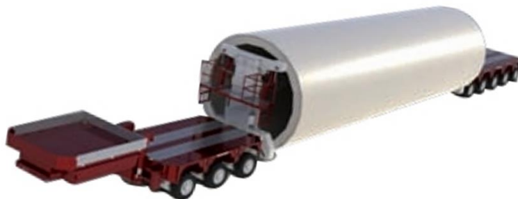
Figure 6.19 Tower adapter mounted directly on the platform
