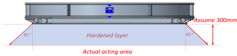
Figure 10.2 Nacelle frame load dispersion sketch
