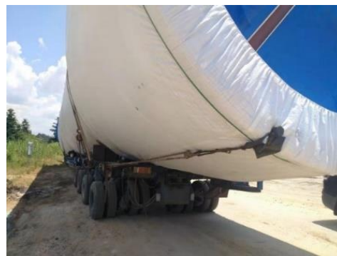
Figure 6.22 Tower lashing in mountainous wind farm
