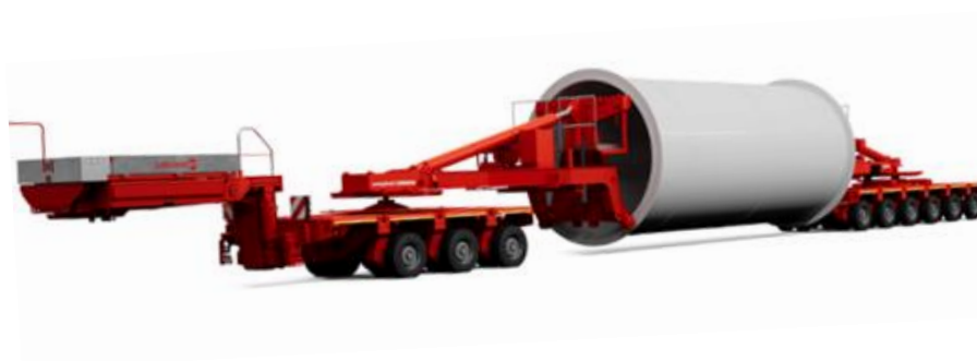
Figure 6.19 Tower adapter mounted directly on the platform
