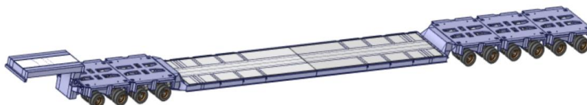
Figure 6.17 Hydraulic trailer with drop deck
