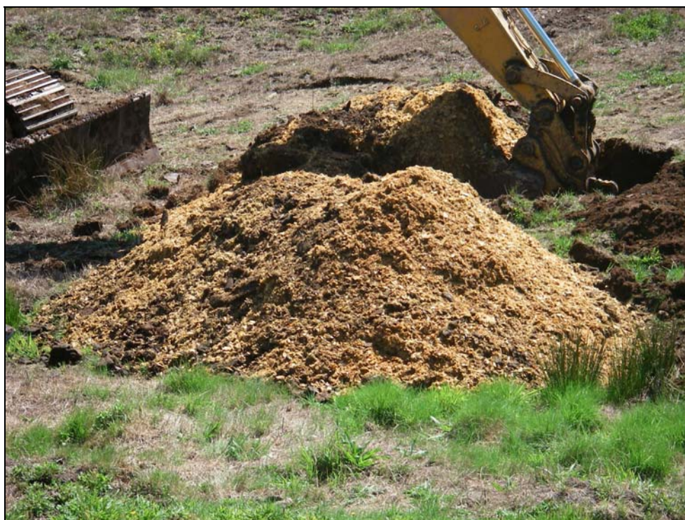
Plate 3: Typical Contents of Test Pits – Sawdust
