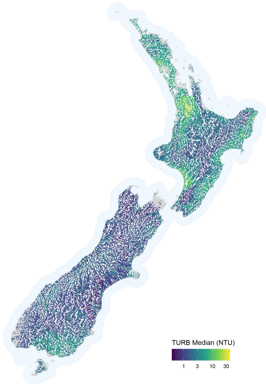
Figure 4-7: Predicted median TURB in New Zealand rivers. Map shows all nzsegments of Order 3 and higher. Values are represented on a \log_{10} colour scale.
