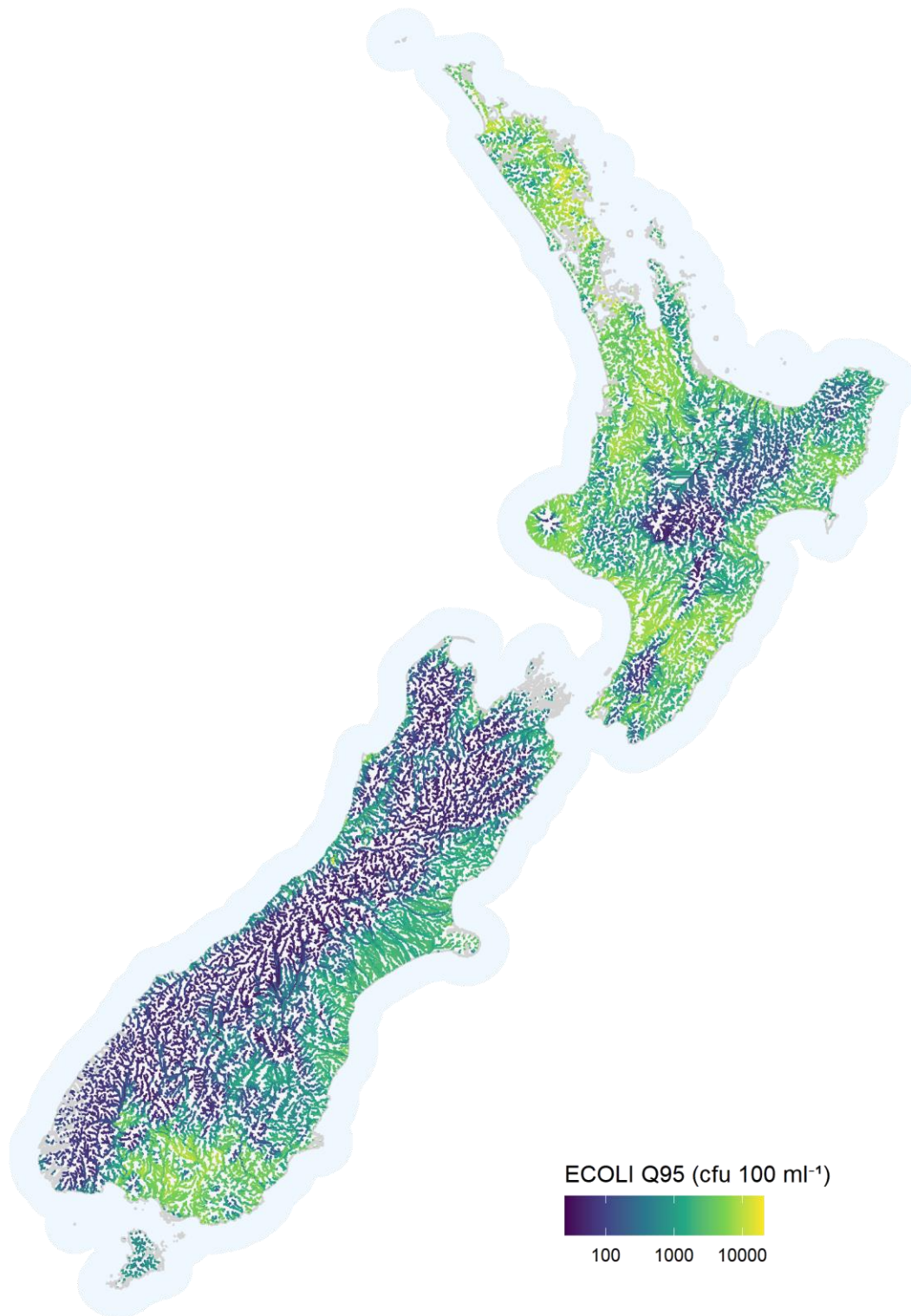
Figure 4-18: Predicted 95 th percentile (Q95) ECOLI in New Zealand rivers. Map shows all nzsegments of Order 3 and higher. Values are represented on a log 10 colour scale.
