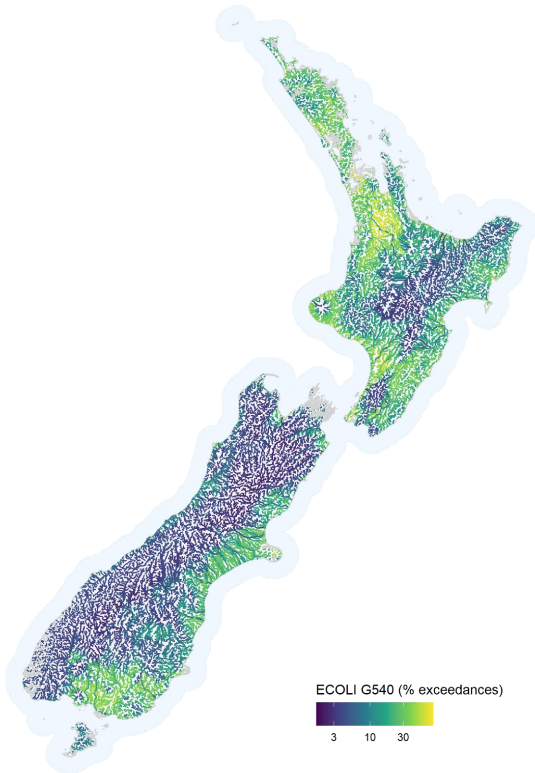
Figure 4-20: Predicted proportion of samples exceeding 540 E. coli 100 ml -1 (G540) ECOLI in New Zealand rivers. Map shows all nzsegments of Order 3 and higher. Values are represented on a log 10 colour scale.
