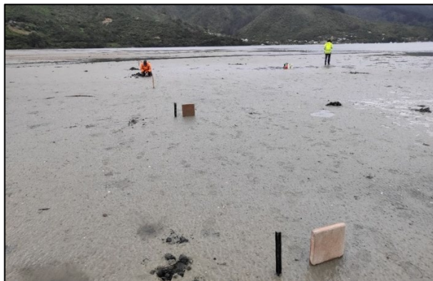
Setting up a site for a transect sediment plate installation using Configuration 2 above.
