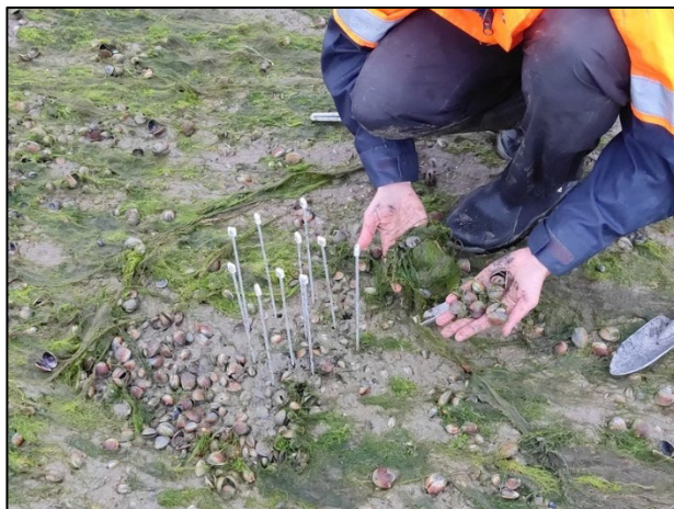
Care is needed in shelly sediments to ensure that the measurement probe penetrates to the plate, and an erroneous depth is not recorded due to the probe hitting shell.
