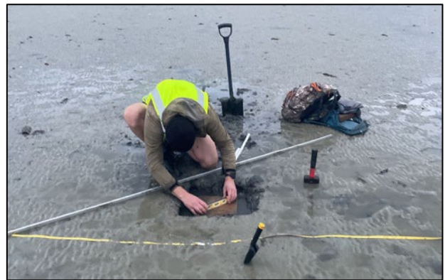
Final leveling of a plate using a spirit level.
