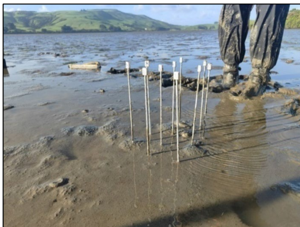
Measuring a buried sediment plate using knitting needles.
