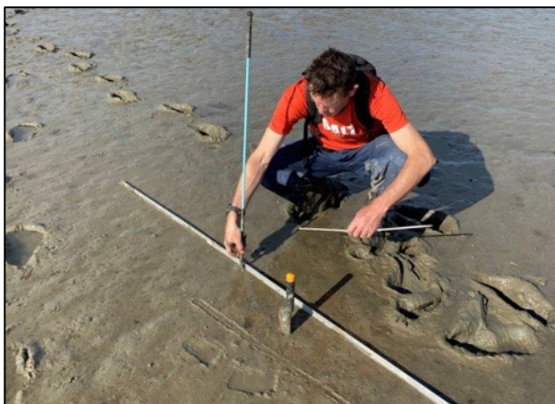
Measuring a buried sediment plate using a fibreglass stock rod (1.1m long) and straight edge.
