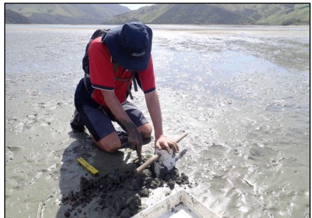
Collecting a macroinvertebrate core. A handle inserted through holes drilled in the top of the corer can be used to rotate it in alternating directions to penetrate the matrix of firm or shelly sediments. A trowel or similar may be needed to dig around the edges to enable corer extraction.
