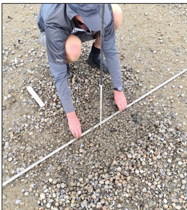
When using a straight edge where there is surface shell, make sure it contacts the sediment surface and is not elevated on top of shell material.
