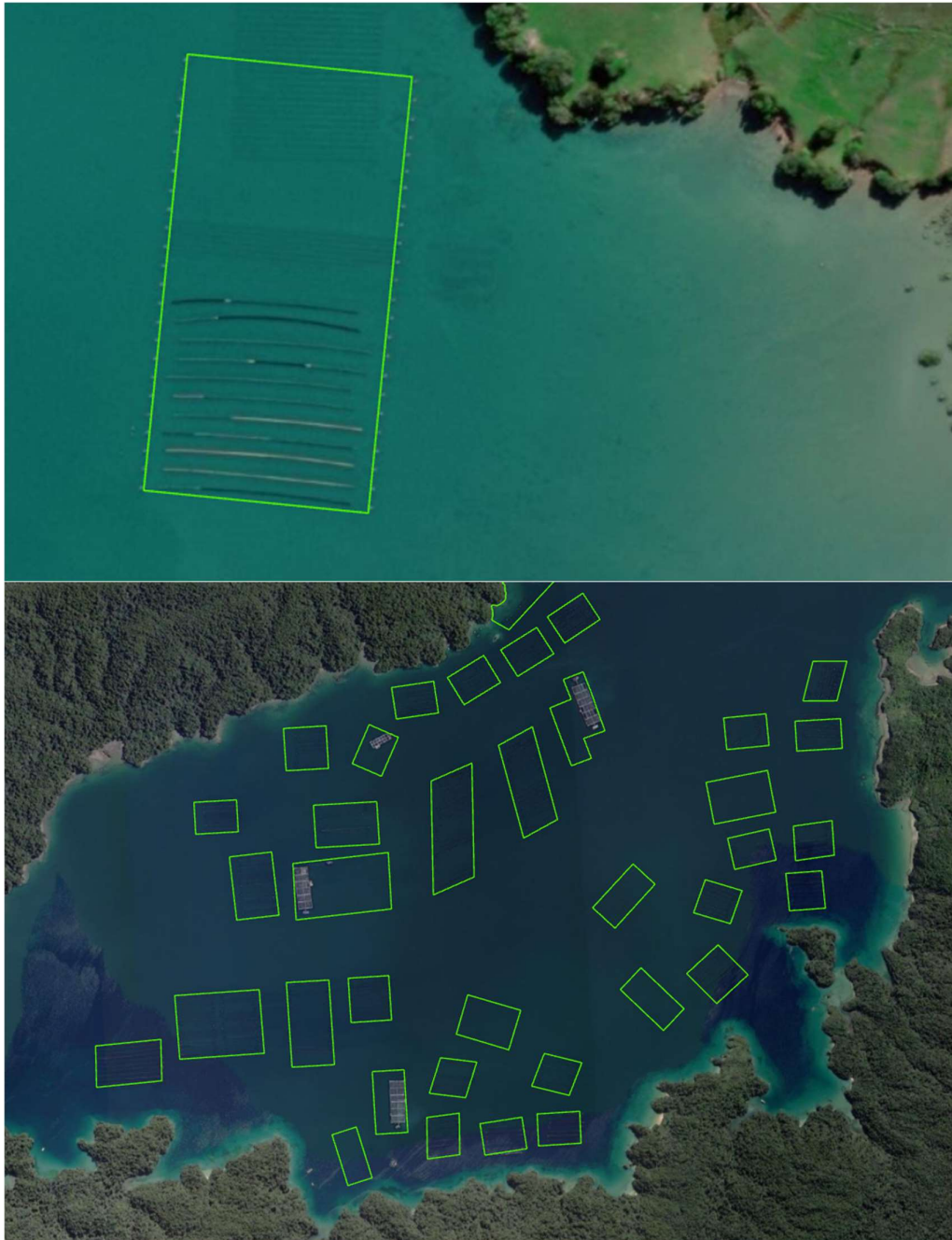
Figure 6-3: Example of validation of proportion of a marine farm being used to quantify the stressor footprint. Suspended shellfish culture lines, Te Kouma, Waikato (top); Salmon farms, Stewart Island (bottom). Green outlines indicate licensed marine farm areas.
