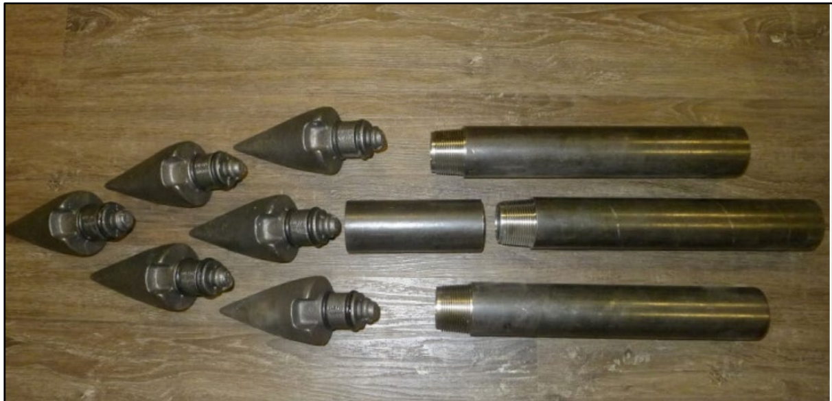
Figure 7 Example of a lost cone and steel casing used for direct push piezometer installation.
