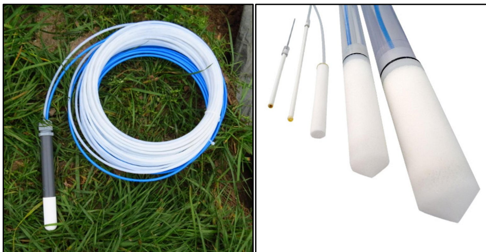
Figure 5 Ceramic suction cup (left), and Teflon suction cup (right) lysimeters for soil water extraction (Ecotech, 2024).
