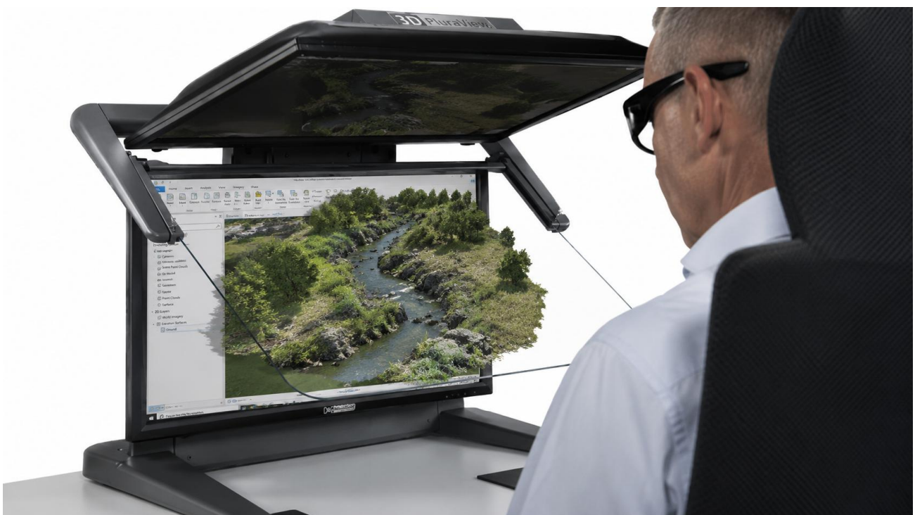
Figure 5. Example of the stereoscopic workstation used for desktop interpretation of overlapping aerial photographs. A dual-screen 3D PluraView display, dedicated graphics hardware, and active shutter glasses provided a three-dimensional view of the stream. (Source: adapted from https://www.geospatialnext.org/workstation-for-gis-and-mapping/ )
