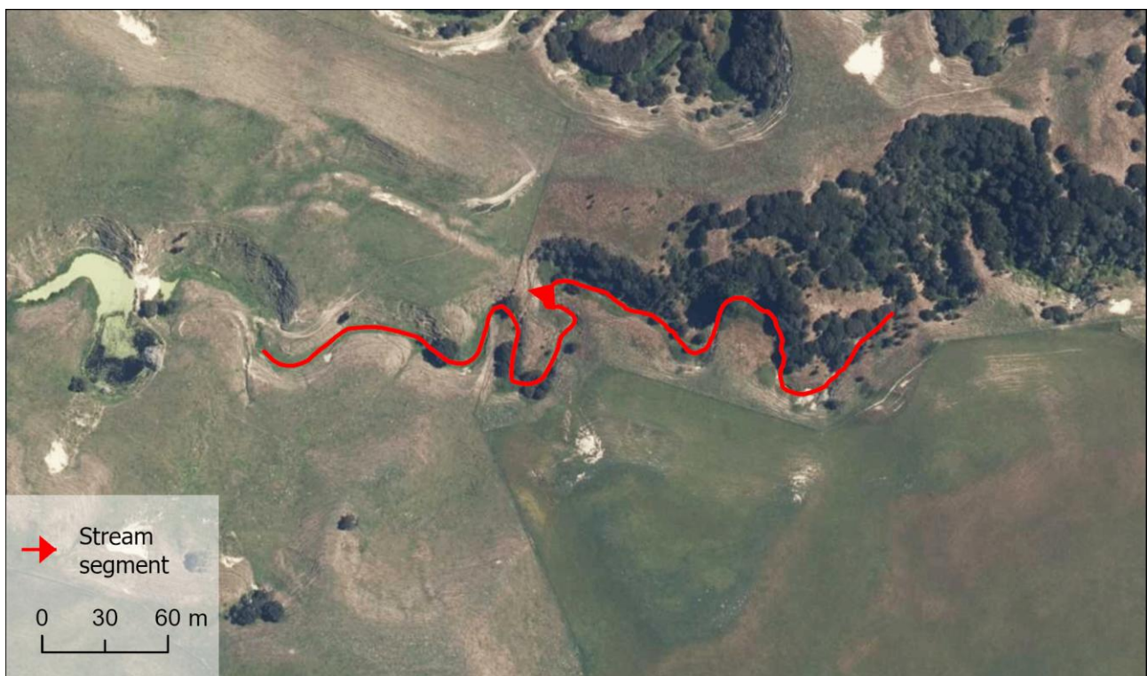
Figure 6. Example of the 25 cm standard resolution orthophotography used for desktop assessment of streambank and riparian characteristics. The red line indicates the surveyed stream reach used for the imagery assessment and the arrow shows the direction of flow.
