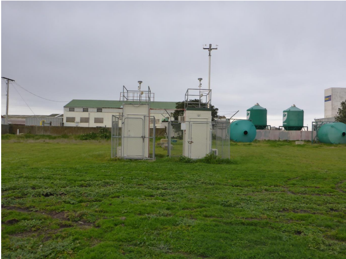
Figure 1.1: HBRC’s air quality and climate site at Waitangi Road, Awatoto. The hut on the left houses a Thermo FH62C14 BAM measuring PM 10 and the hut on the right houses a Thermo FH62C14 BAM measuring PM 2.5 . The mast with climate instruments is adjacent to the hut on the right.
