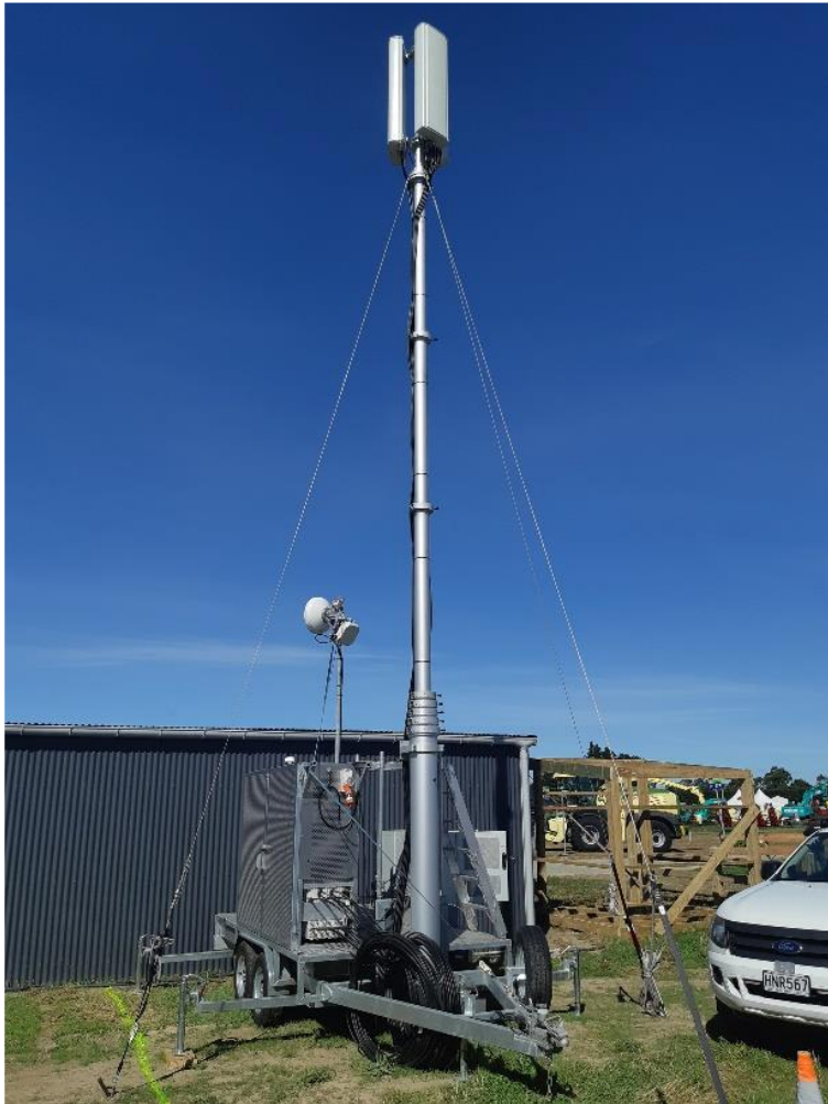
Figure 7: Example of a temporary telecommunication facility known as a 'cell-on-wheels' attached to a trailer (provided by Spark)
