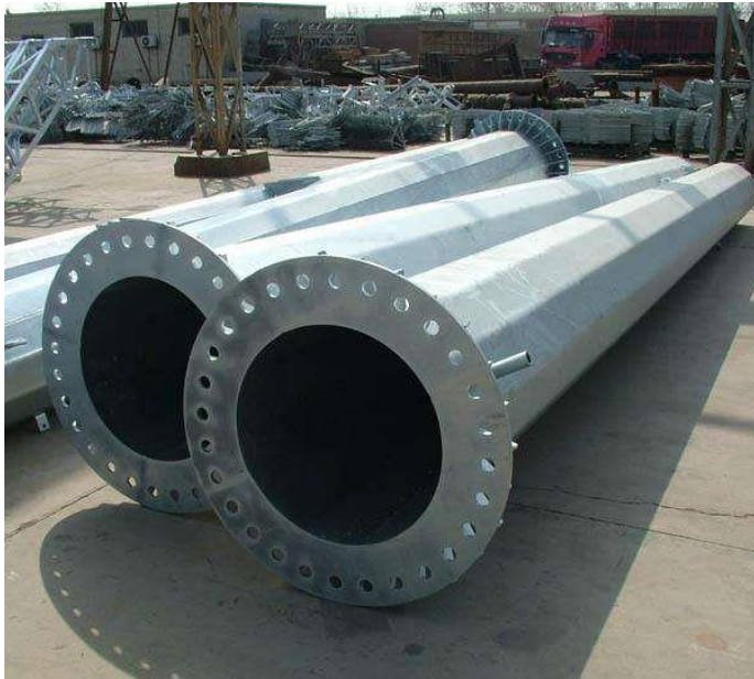
Figure 8: Flange or projecting part at the base of the pole excluded from pole width measurements
