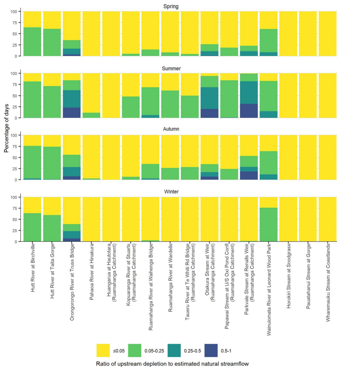
Figure 17: Percentage of spring, summer, autumn and winter days where the ratio of upstream depletion to estimated natural streamflow exceeded thresholds at gauging sites in the Wellington region, June 2015–May 2018
