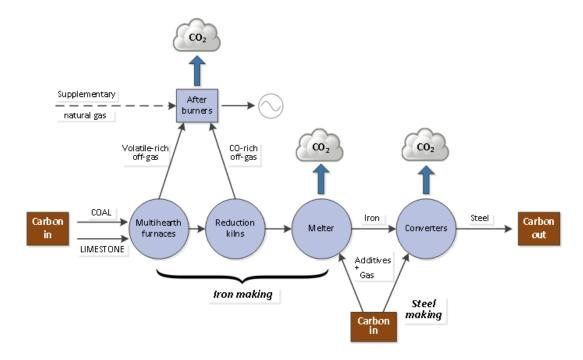
Nearly all the carbon entering the process is from coal used as a reductant in the iron-making process, and nearly all of this is emitted as  $CO_2$  in two waste gas streams:
