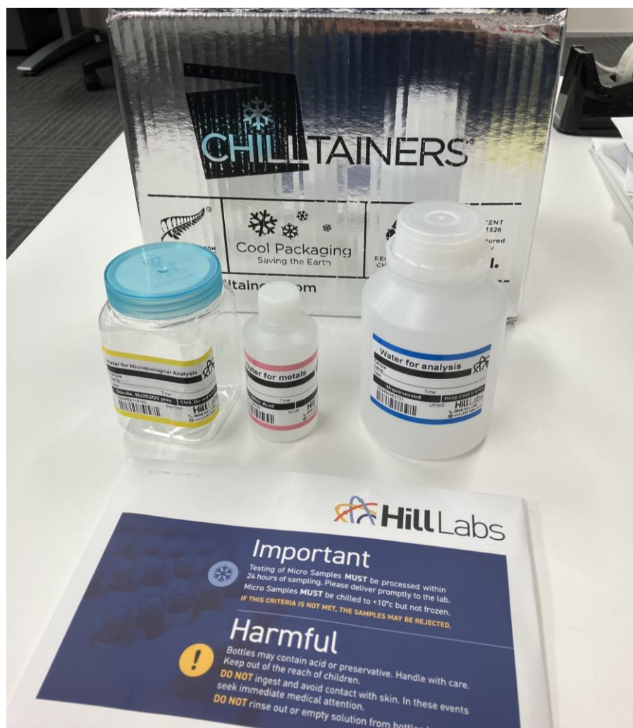
Figure 7.2 Water sampling kit sent by Hill Laboratories to each school.
