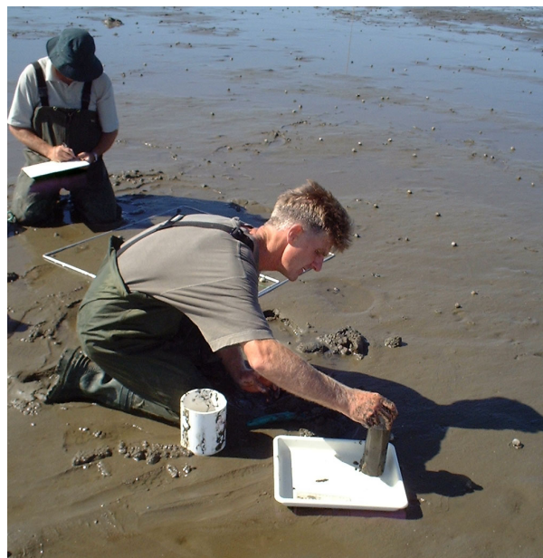
Fine-scale sampling at the New River Estuary, showing the collection of sediment core samples.
