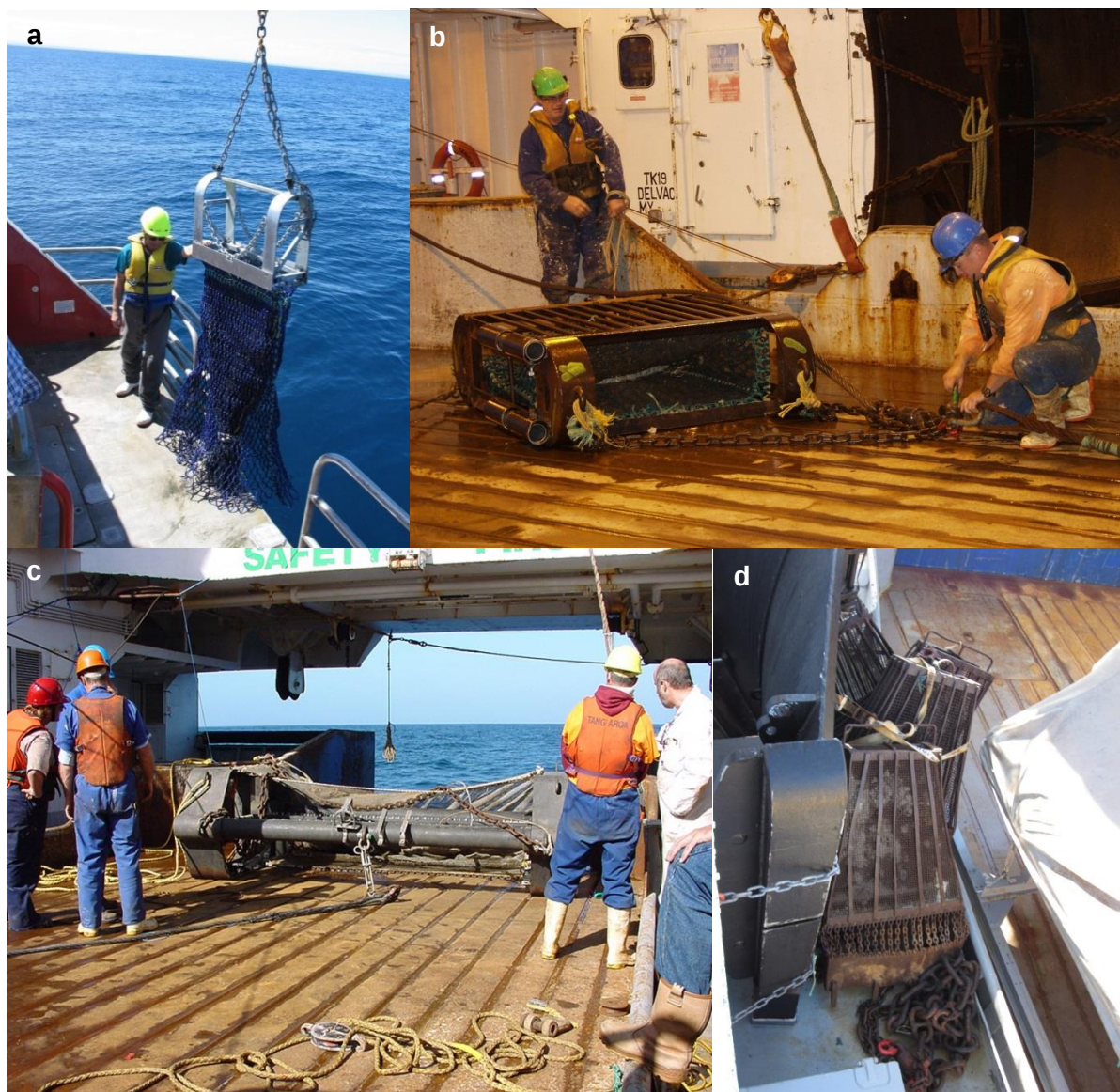
Figure 6-3: Mobile sampling of the seabed. (a) small epibenthic sled, (b) large epibenthic sled, (d) Agassiz beam trawl, (e) rock dredge and spares on RV Tangaroa (all images NIWA).
