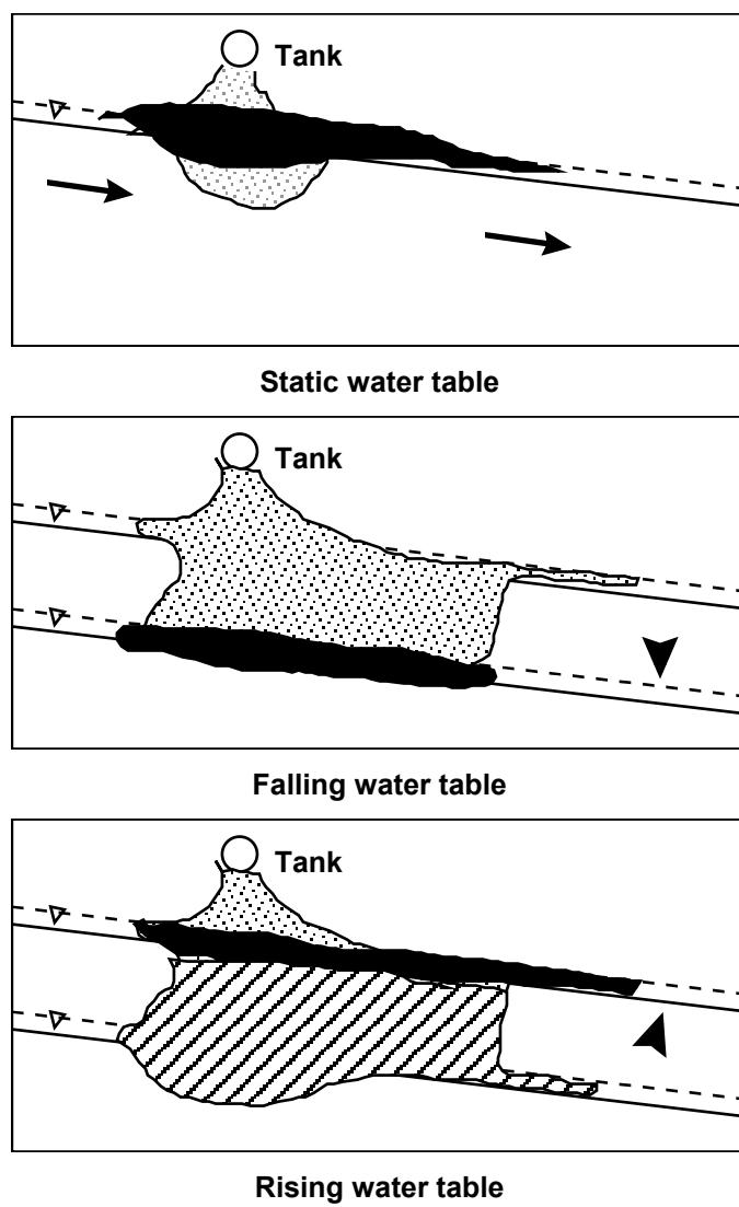
**Figure 2.9 Spreading of hydrocarbons as a result of water table fluctuations**
