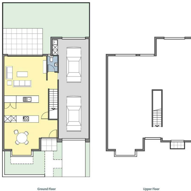
Figure 13: Ground floor plan of terrace houses in Stonefields
