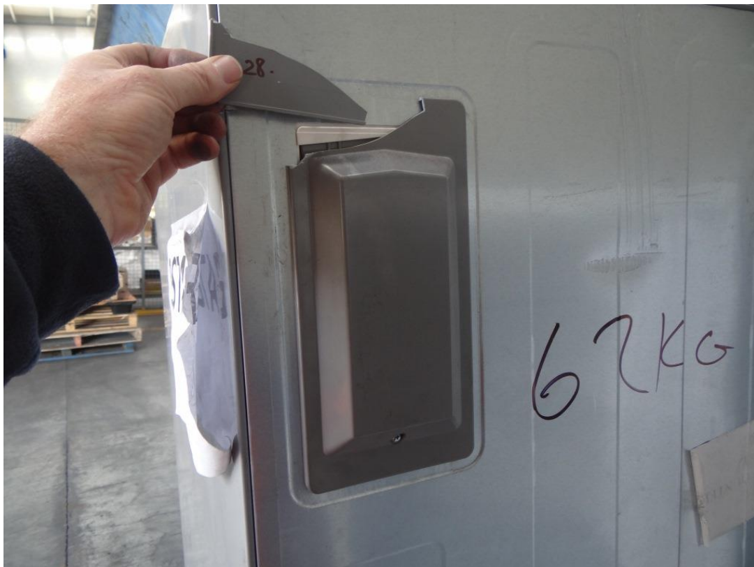
Figure 5: Electrical cover on rear of fridge
