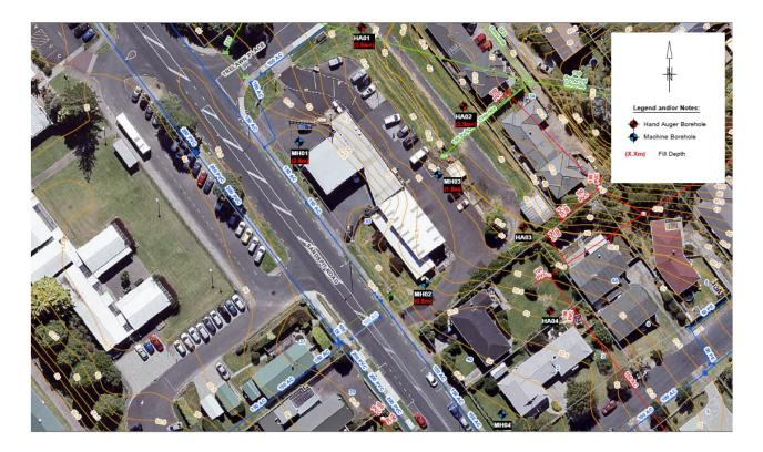
The site is underlain by the East Coast Bays Formation of the Waitemata Group geology. The East Coast Bays Formation consists of alternating sandstone and siltstone beds with varying volcanic and volcaniclastic content. Surficially these deposits typically weather to orange, brown and grey clays, silts and sands.
