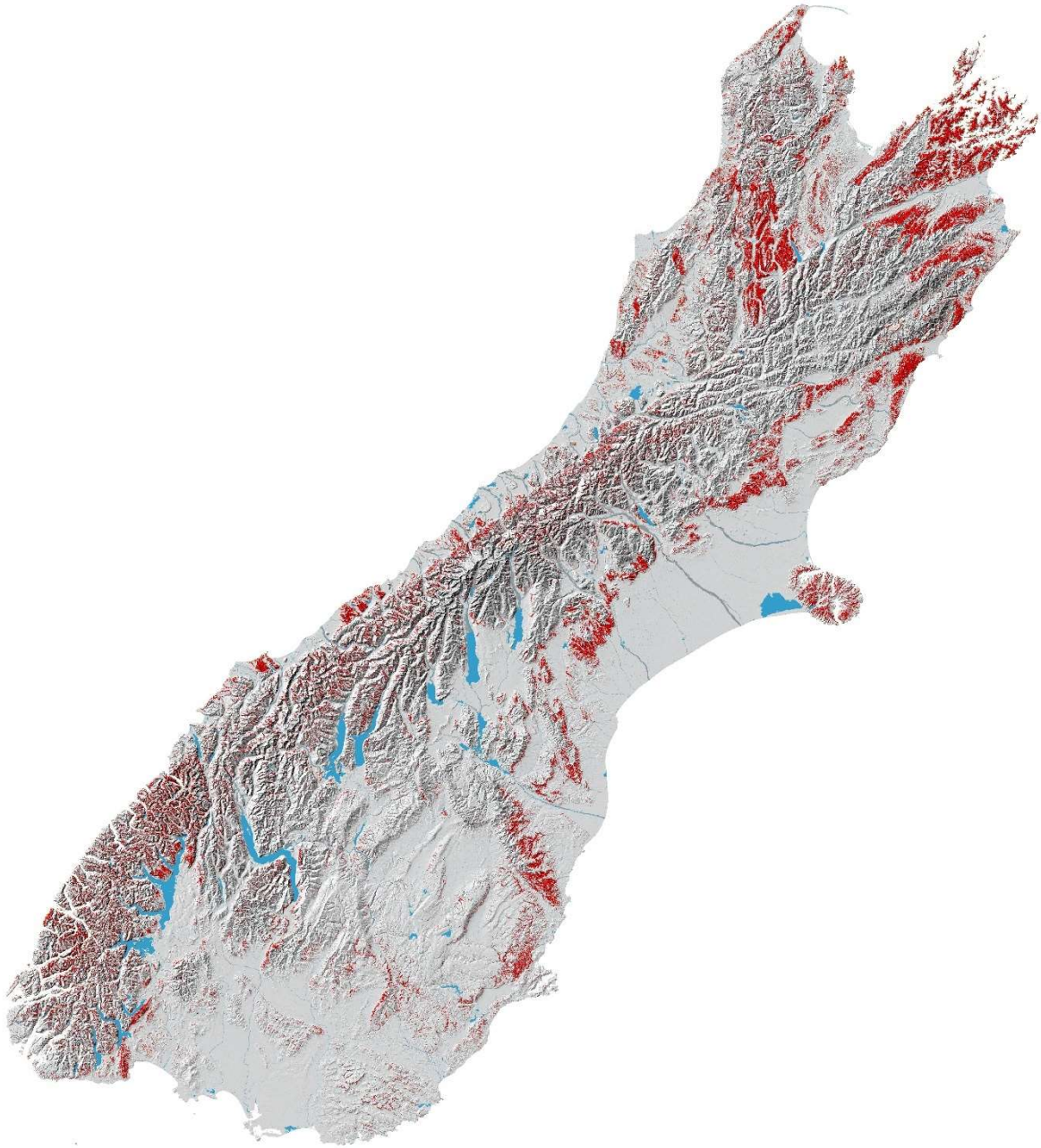
Figure 2. Graphic of fundamental HEL layer of South Island. (Red: high landslide risk – delivery to stream; Light brown: landslide risk – non-delivery to steam; Magenta: moderate earthflow risk; Purple: severe earthflow risk; Orange: gully risk; Green: woody vegetation.)
